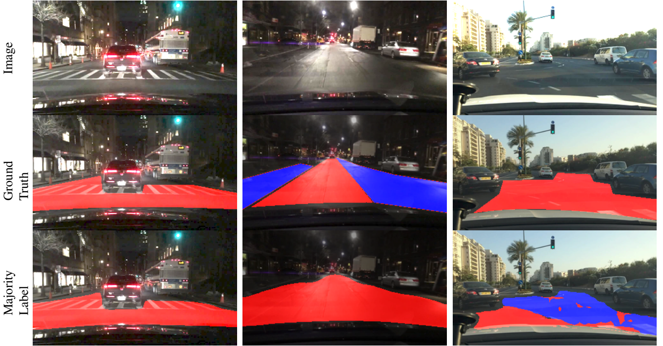
Fig. 3: On the left, we see a three lane one-way street labeled completely as drivable ego area in red. In the center a similar street is labeled as three different lanes, blue marking other drivable area. In variation from the label, the complete street is predicted by the networks as ego lane. On the right side, an inner roundabout lane has a large label for drivable ego area. The group of networks identified some areas which are potentially not part of the ego roundabout lane marked in blue.
